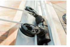
Self-tacking traveler with double self-aligning cars for jib and stay sails.
