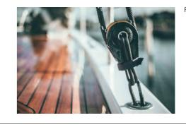
Pad eyes allow slack lines to be kept off deck.
