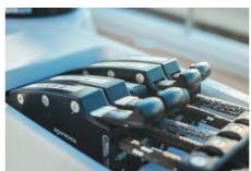
Lines pass through Spinlock jammers and an organizer for precise line handling with a single winch.
