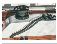
All lines are led aft to keep the large owners and guest area unobstructed. The electric or hydraulic winches have foot controls and a large space for loose lines keeps things organised on deck.
