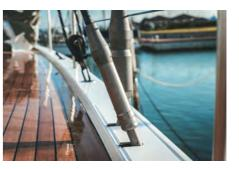
The bulwark is moulded with all local reinforcements and recesses for pad eyes and stanchions for a clean look and minimal obstruction.
