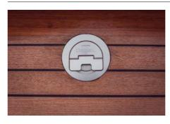
All deck filling points are recessed into the deck.
