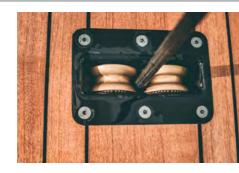
The main sail sheets can be controlled manually or as in this case by means of a magic trim. The image shows the passage of the sheets under the custom designed deck.
