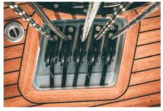
A clean solution for the mast-foot blocks which are recessed, allowing sheets to pass below deck for minimal obstruction.
