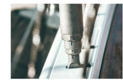
Special attention has been paid to the shroud terminals of the diagonal and vertical stays which are mounted to chain plates hidden within the hull sides.
