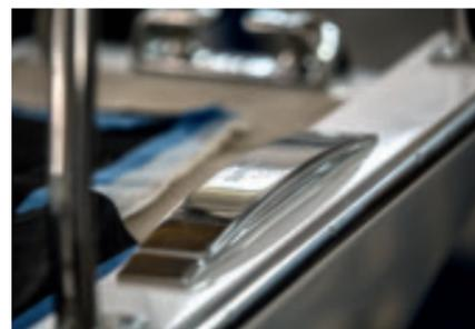
The recessing cleats are equipped with highly resistant stainless steel or carbon chaffing plates.
