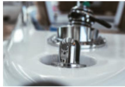
The code-0 furler is recessed in the bow on a special plate giving maximum strength and optimal inclination.
