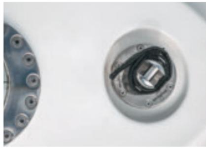
Only the strongest furlers are installed on board using a special fastening assembly.
