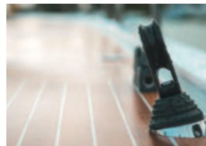
The deck block angle is optimized by the use of custom plates.
