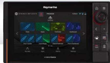
Raymarine AXIOM PRO 9 S chart plotter with HybridTouch multifunction display at helm station, ps
