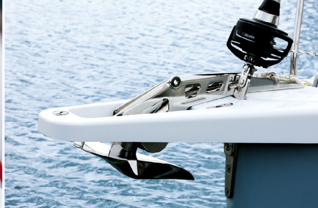
The optional bow sprit increases the sailing performance with asymmetrical headsails.
